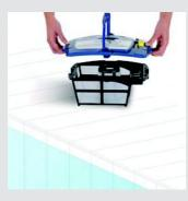
Press the two buttons located below the sides of the lid. Pull the handle and remove the cover.
