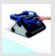
Press the Push'n' $Go^{TM}$  button, located on the top of the cleaner, to release the handle of the filter basket.
